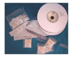
Based on a novel polymer PCM system, this material exhibits excellent wetting at interfaces during typical operating temperature range, resulting in very low surface contact resistance.
