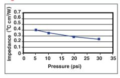
Key outputs in thermal impedance for PCM45F have been measured to fit individual needs.
